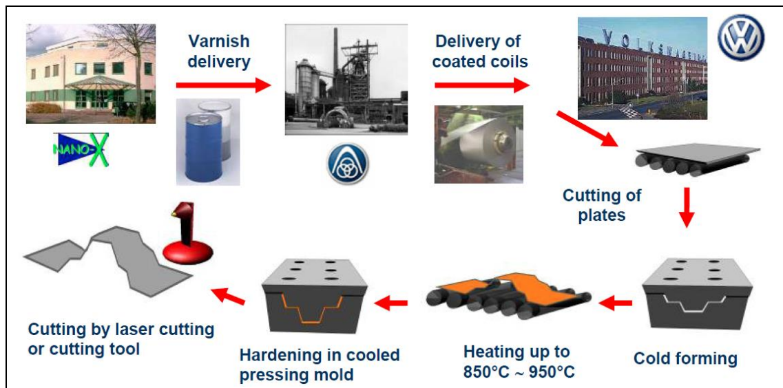
Figure 14: A NANO-X anti-scaling product (x-tec® CO 4017) introduced for a new process at VW for structural body parts and safety parts of VW cars [Sepeur 2006a].
